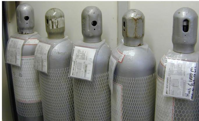
**Figure 13 – Cylinder Gases Used for Calibration**
